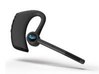
The new BlueParrott M300-XT with its comfortable new design addresses these challenges head-on. The Bluetooth mono-headset is the smallest and lightest BlueParrott headset, weighing in at just 0.7 oz/20 g. Especially designed for noisy environments, the M300-XT has an unparalleled 80 per cent of noise cancellation with its 2-microphone technology, creating a clear communication with no annoying sound interruptions, wherever you're calling from.
